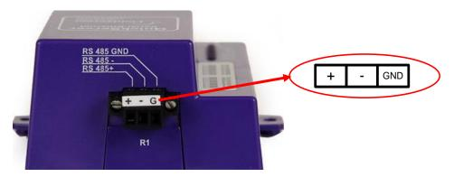
The following Baud Rates are supported on the R1 Port: 110, 300, 600, 1200, 2400, 4800, 9600, 19200, 20833, 28800, 38400, 57600, 76800, 115200
