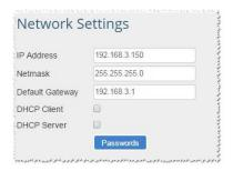
The IP settings for the Router are also used by both BACnet/IP connections. The IP settings can be changed in the Network Settings section as shown.
