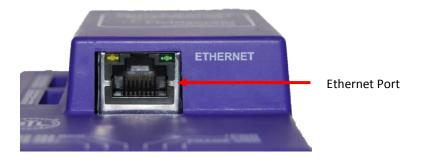
The Ethernet Port is used both for BACnet Ethernet and BACnet/IP communications. It is also used for configuring the Router from a Web page. Follow the steps below to connect the Router to a BACnet network and optionally to a PC for configuration purposes:
