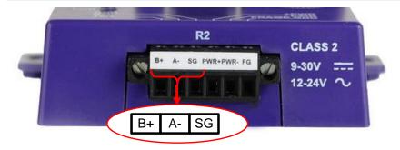
Connect to the 3 pins on the left-hand-side of the 6 pin connector as shown.
